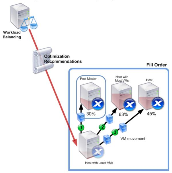
This illustration shows how, when consolidating VMs on hosts in Maximum Density mode, XenServer® fills the pool coordinator first, the most loaded server second, and the least loaded server third.
